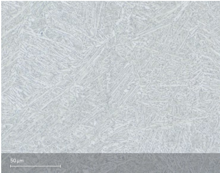
Heat treated microstructure. Etched according to ASTM E407 modified recipe #190.
