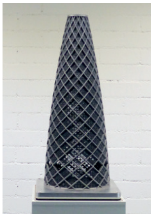
Fig 1: AlSi10Mg demo part 1.000mm height, Ø 380mm, Build time: ~ 73 hours
