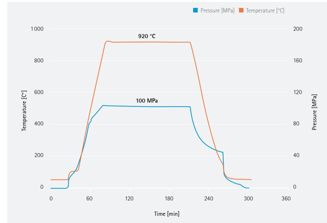
Figure 7a: Standard HIP cycle for titanium alloys (920 °C, 100 MPa, 2 h)
