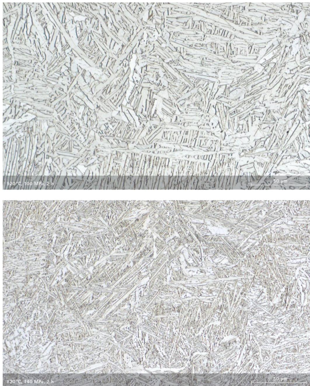
Figure 8. Microstructure of LPBF Ti64 material HIPped with standard HIP parameters (920 °C, 100 MPa, 2 h) and with optimized HIP parameters (820 °C, 140 MPa, 2 h).
