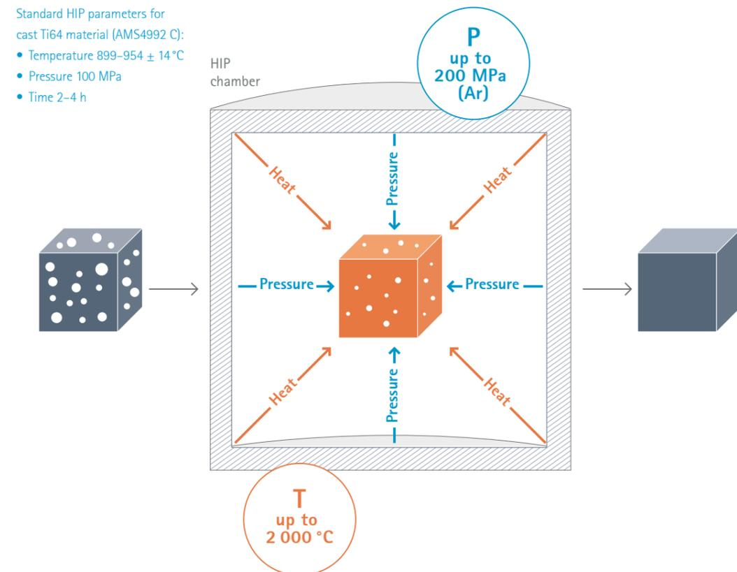
Figure 1. Principle of material densification by Hot Isostatic Pressing (HIP)
