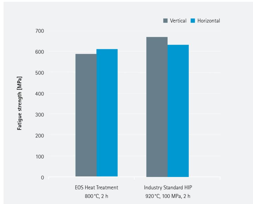
Figure 2. Fatigue strength ( $10^7$  cycles) of EOS Ti64 HiPer 40 µm material in heat treated state and HIPped with industry standard parameters show only a minor difference
