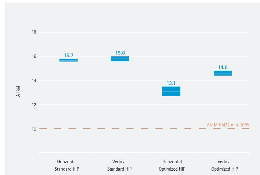
Figure 9. Mechanical properties of Ti64 material post-treated with optimized HIP cycle (820 °C, 140 MPa, 2 h) compared to properties reached with current industry standard HIP cycle (920 °C, 100 MPa, 2 h). Yield strength is higher with the optimized HIP cycle compared to standard HIPping. Elongation is slightly lower but well over the limit of the material standard (ASTM F1472, N=9 or N=11). Average results with 95 % confidence limits.
