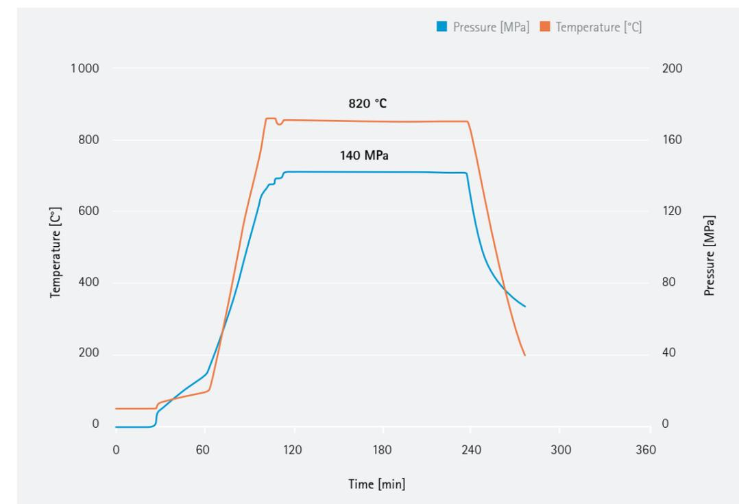
Figure 7b: Optimized HIP cycle for LPBF Ti64 (820 °C, 140 MPa, 2 h)
