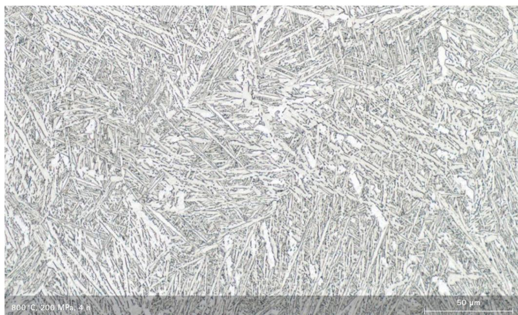
Figure 6. Effect of HIP time on the microstructure of LPBF Ti64 material. Slight lath growth observed with longer HIP time
