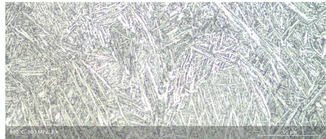
Figure 5. Effect of HIP temperature on the microstructure of LPBF Ti64 material. A smaller lath size is reached with lower HIP temperature
